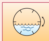
DRUMS: The major vessel used in leather processing.
